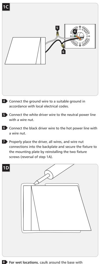
• For wet locations, caulk around the base with waterproof construction sealant.
