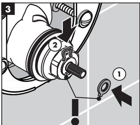
\*\*To prevent scald injury, the maximum output temperature of the shower valve must be no higher than 120°F. In Massachusetts, the maximum output temperature can be no higher than 112° F.
