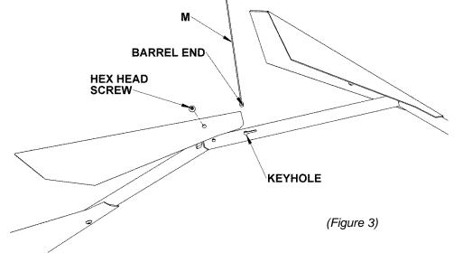
5. Screw cable gripper (P) back on to gripper base. Insert support cable (M) into cable gripper. With the swivel portion of the cable gripper oriented horizontally adjust support cable to correct height. Using heavy duty cable cutters, cut excess support cable (M) short enough to allow swivel to rotate.
