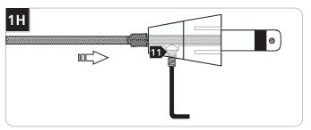
11) Firmly tighten the set screw on the conical connector.
