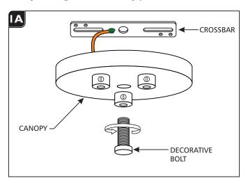
Remove the crossbar from the canopy by completely unscrewing the decorative bolt.
