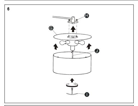
6. Connect the fixed lamp support (G) set into the arms socket and tighten with the nuts (H). Fix the lamps and the screen. Introduce the hilt (I) into the axle switch (J) and tighten it to a firm support.
