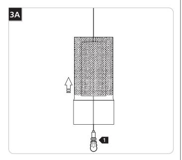
1 Lift both glass shades up to expose the socket.
