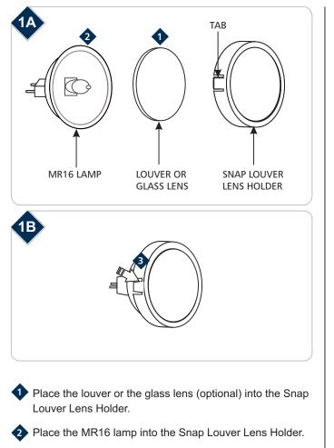
Press the tabs on both sides of the Snap Louver Lens Holder against the MR16 lamp to keep it in the position.
