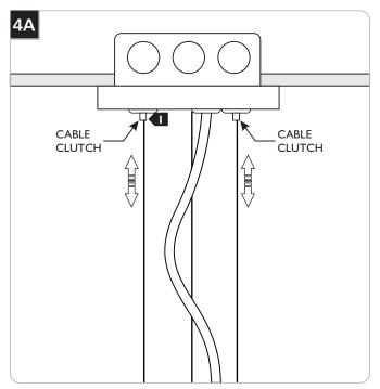
1 If necessary, adjust the aircraft cables until the fixture is level; feed the cable into the cable clutch to raise the fixture and push in on the cable clutch nipple to release the cable and lower the fixture.
