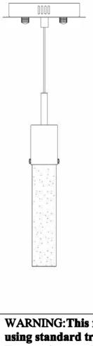
WARNING: This fixture may be dimmed using standard triac dimmer. For maximum adjustability We recommend Lutron CL series dimmers.
