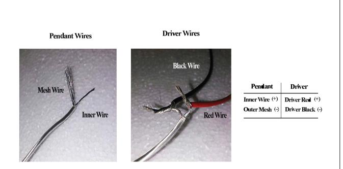
If wires are cut in the process of adjusting the height, please note the pendants consist of an Step 3. outer mesh (ground) and inner (live) wire that must be seperated before rejoinging to driver
