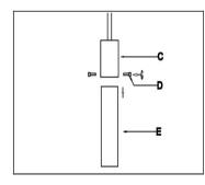
Step 5. Insert glass (E) into cup (C) and secure using screws (D) provided
