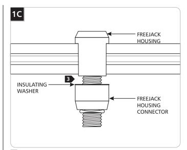
Ensure the spacing of the connectors are correct and tighten the FreeJack housing connectors to the FreeJack housings.
