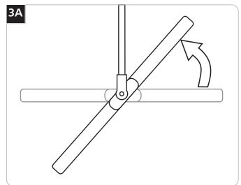
**1** Rotate the panel to the desired position.
