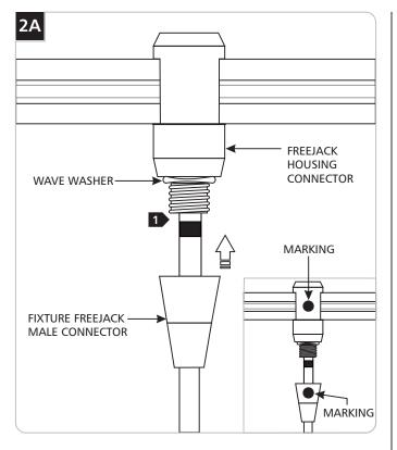
Push and screw the fixture FreeJack male connectors all the way into the FreeJack housing connectors. Make sure to match the FreeJack male connector marked with the black dot to the FreeJack housing connector with the same marking. **Adjust the Fixture**
