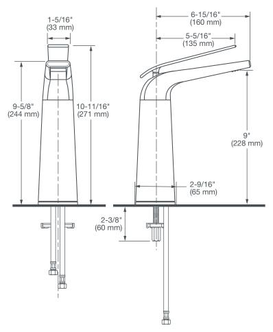
NOTE: MOUNTING HOLES ARE 1-3/8" D. (35 mm)
