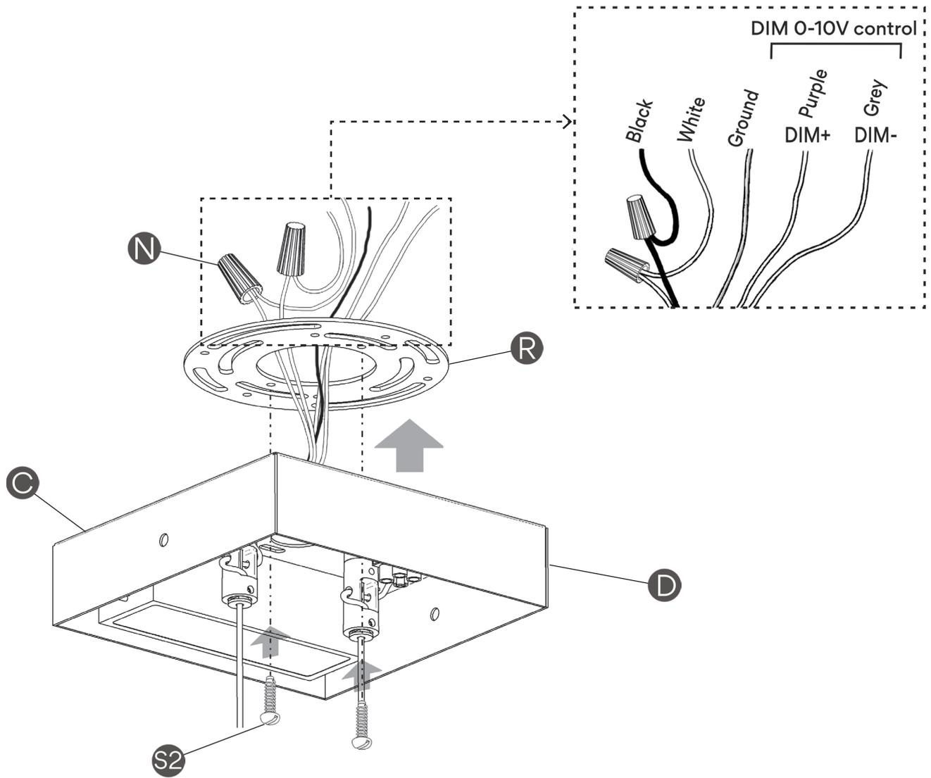
**IMPORTANT:** You have ordered a fixture with a driver specifically compatible with 0-10V DIMMING SYSTEM. This fixture will not be compatible with other types of dimming systems. You can check you have the correct product by looking at the model number printed on the box label or fixture canopy: 2500-XX/12, 2501-XX/12 and 2502-XX/12.
