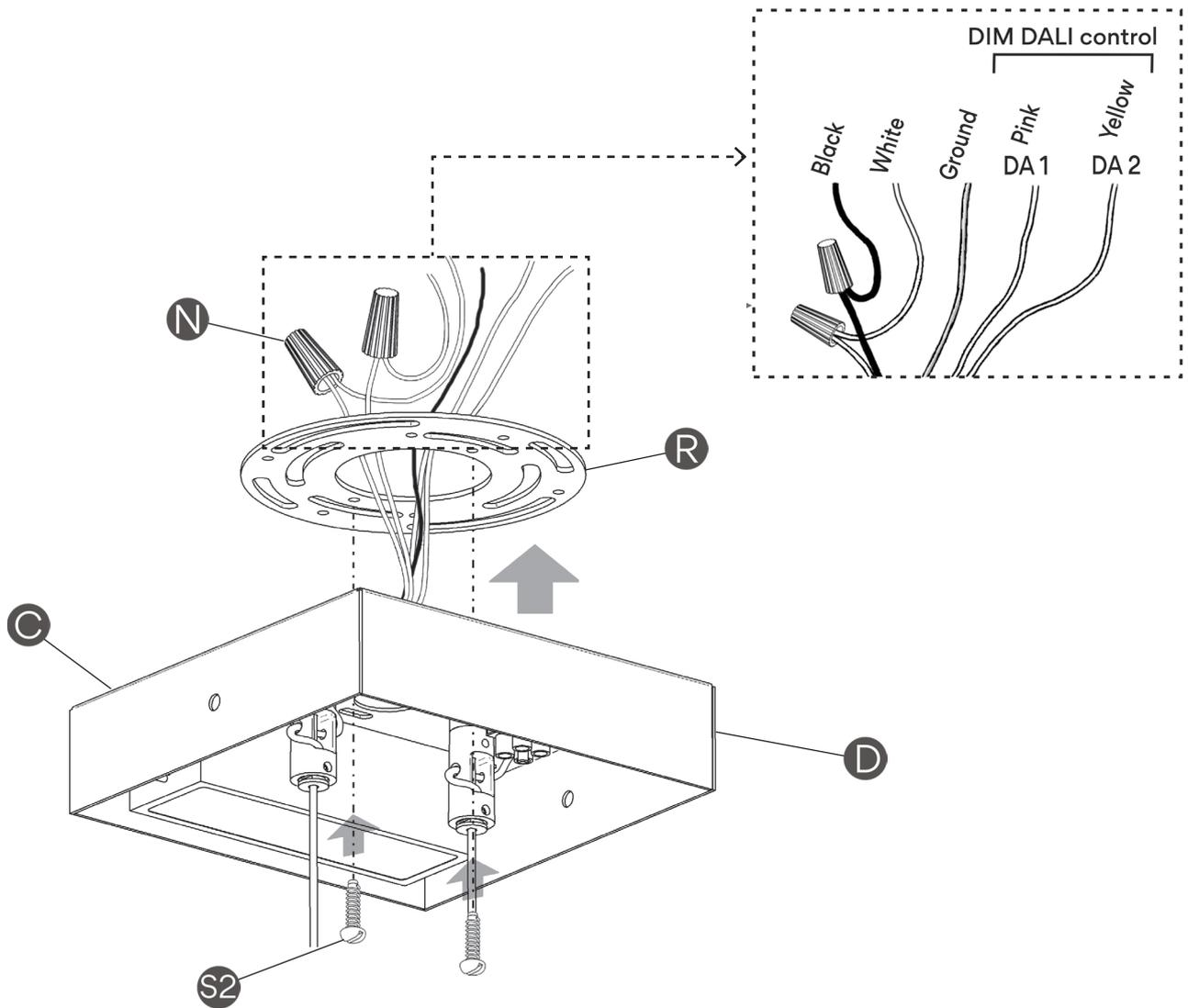
**IMPORTANT:** You have ordered a fixture with a driver specifically compatible with DALI DIMMING SYSTEM. This fixture will not be compatible with other types of dimming systems. You can check you have the correct product by looking at the model number printed on the box label or fixture canopy: 2500-XX/11, 2501-XX/11 and 2502-XX/11.
