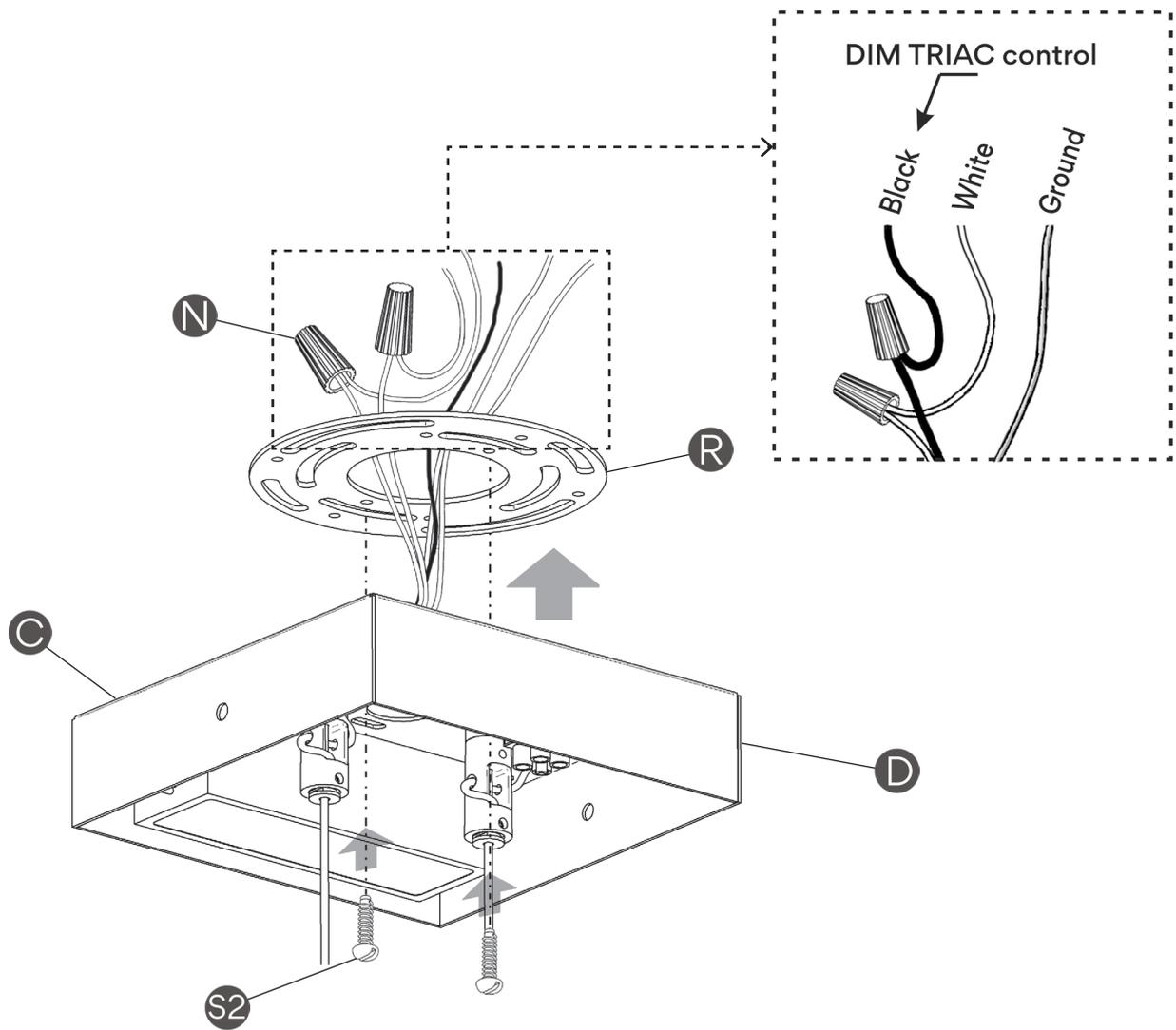
**IMPORTANT:** You have ordered a fixture with a driver specifically compatible with TRIAC DIMMING SYSTEM. This fixture will not be compatible with other types of dimming systems. You can check you have the correct product by looking at the model number printed on the box label or fixture canopy: 2500-XX/14, 2501-XX/14 and 2502-XX/14.
