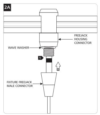
1 Push and screw the fixture FreeJack male connector all the way into the FreeJack housing connector.
