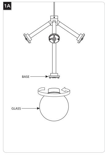
1 Install the glass by screwing it into the base. **Do not** over-tighten.
