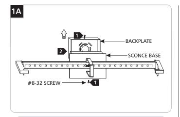
**CAUTION:** When handling the fixture, do not apply pressure to the LEDs. Hold the fixture by the sconce base only.
