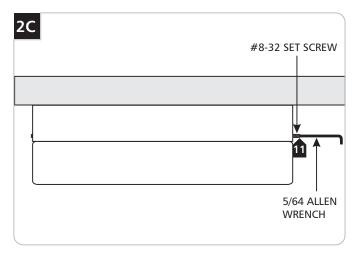
Tighten the two #8-32 set screws with the 5/64 Allen wrench.
