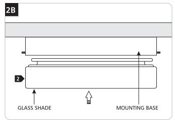
Push the glass shade completely into the mounting base until it snaps properly into the springs.
