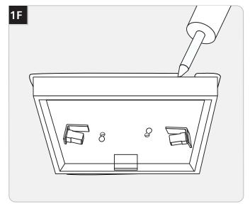
**9** For wet location installation, caulk around the mounting base with waterproof construction sealant.
