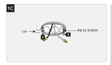
Thread (NOT COMPLETELY) the two #8-32 screws into the electrical box holes leaving 1/4" of them exposed.
