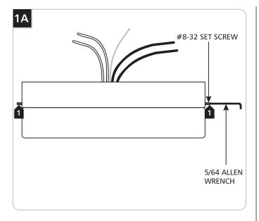
Back out (**DO NOT REMOVE**) the two #8-32 set screws for 1/4" with the 5/64 Allen wrench.
