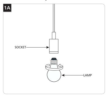
**CAUTION:** To reduce the risk of a burn or electric shock during relamping, disconnect the power to the fixture.
