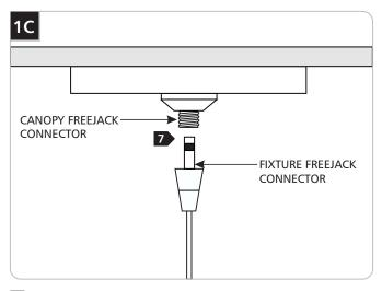
Screw the Fixture FreeJack male connector into the FreeJack female connector.
