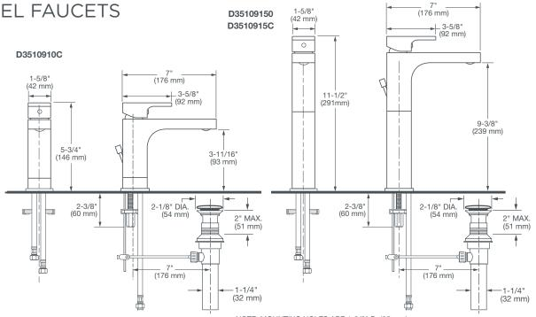
NOTE: MOUNTING HOLES ARE 1-3/8" D. (35 mm)
