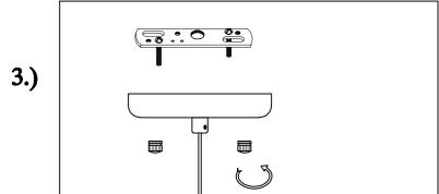
Step.3: Screw finials (D) onto mounting bracket (A) until canopy is flush with ceiling. Adjust the wire to desired length according to Page 3.
