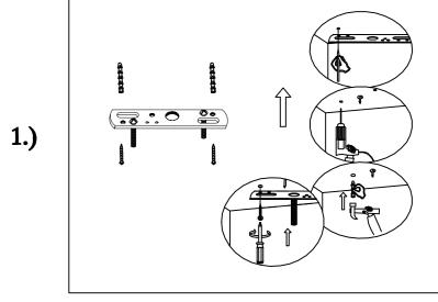
Step.1: Remove mounting bracket (A) from Canopy (C) to install to electrical box
