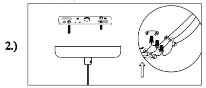
Step.2: Wire fixture to wires in outlet box. Green wire is for Ground.
