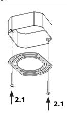
2. Engage the two screws (supplied) into the mounting plate.
