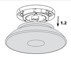
1. Fix the mounting plate to the J-Box (screws not supplied).
