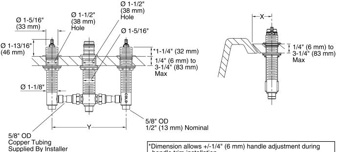
\*Dimension allows +/-1/4" (6 mm) handle adjustment during handle trim installation.
