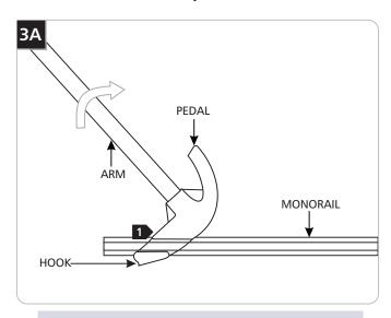
**NOTE:** The Wiremold pipe bender can be used to create smooth horizontal curve of 90° or less. Avoid stepping on the pedal of the pipe bender which will flatten and damage the MonoRail.
