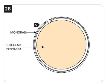
5 Start bending the rest of the MonoRail against the circular plywood until the desired curve or circle is achieved.
