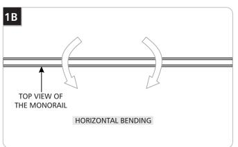
NOTE: There are three techniques to bend the MonoRail horizontally, Plywood Template, Wiremold Pipe Bender, and Freestyle. When bending the MonoRail vertically, only use the wiremold pipe bender technique. MonoRail bends horizontally easier than vertically. When bending the MonoRail vertically, do small bends at the time and avoid bending the MonoRail back which may cause the rail to separate from the insulator.
