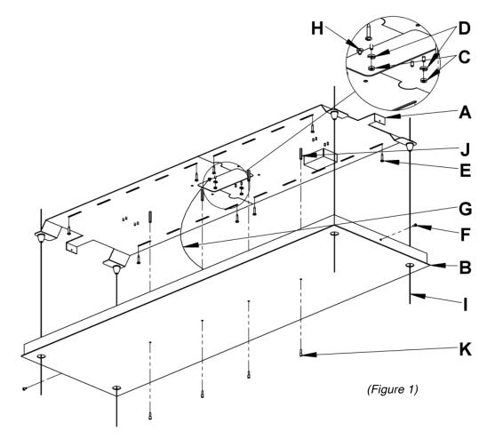
4. Raise canopy (B) close to ceiling and attach safety cable (G) using safety cable nut (H) that is shipped installed in the mounting bracket (A).
