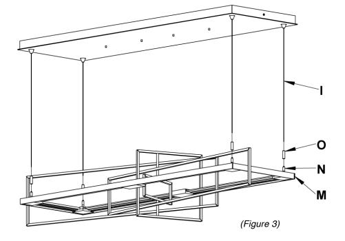
1. Insert supply cable (I) through gripper cover (O) and into gripper (N) until cable (I) sticks through the slot in the side of the gripper (N).
