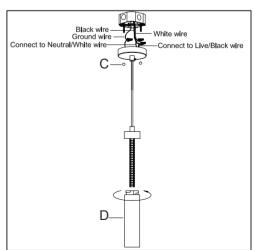
Step2:Wire fixture to wires in outlet box. Copper wire is for Ground. Attach canopy to mounting bracket and tighten with ball nuts.
