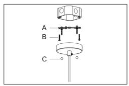
Step1:Remove mounting bracket from fixture and install to electrical box.
