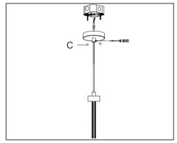
Step2: Adjust wire length to desired mounting height, and tighten strain relief screws to secure.
