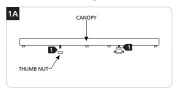
Separate the mounting plate from the canopy by first unscrewing and removing the two thumb nuts.
