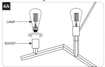
**CAUTION:** To reduce the risk of a burn or electric shock during relamping, disconnect the power to the fixture.
