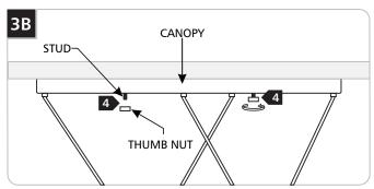
Re-install the canopy by aligning the studs of the mounting plate to the holes in the canopy and secure it in place with the two thumb nuts.
