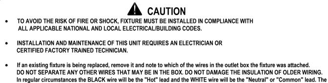
GREEN or BARE COPPER wire is the "Ground". In older buildings it is always good practice to reconfirm the polarity of the wiring.
