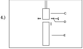
Step 4: Insert glass (E) into cup (C) and secure using screws (D) provided.
