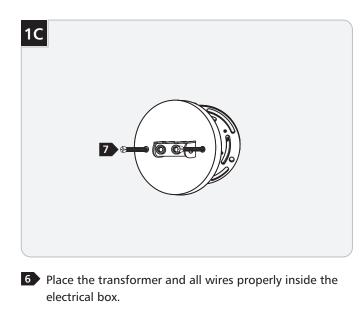
7 Mount the 4" round canopy to the electrical box with two long #8-32 screws provided.
