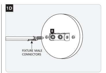
8 Push the two fixture male connectors all the way into the Display Jack ports.
