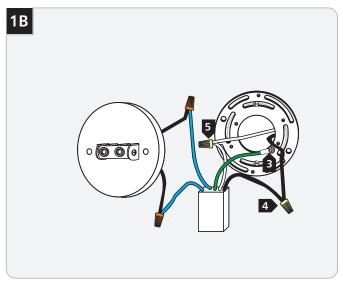
Connect the green ground wire according to electrical code of the region.
